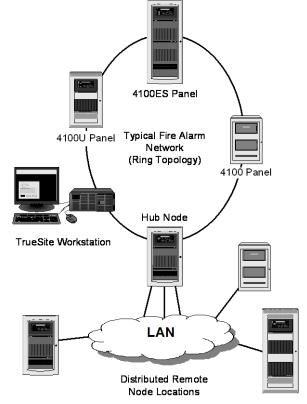
4120 Network with TCP/IP Interconnection of Hub Node to Star Connection
